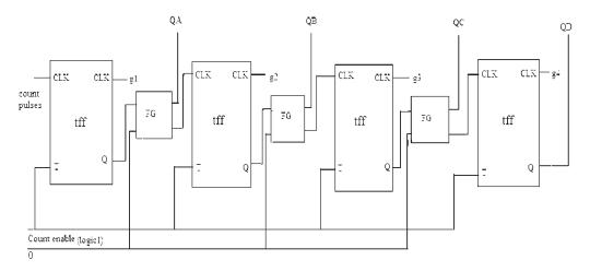
Fig. 5: Block diagram of reversible asynchronous down counter
