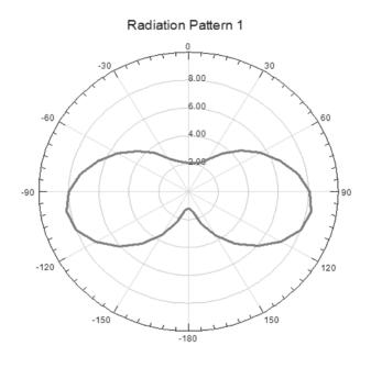
Figure 5: Radiation Pattern at 4.20 GHz
