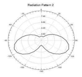
Figure 6: Radiation Pattern at 4.40 GHz
