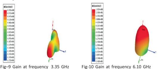
Fig-9 Gain at frequency 3.35 GHz
