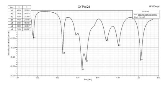
Figure 3: Return Losses or S-Parameter
