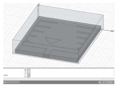
Figure 1: Geometry of Proposed antenna
