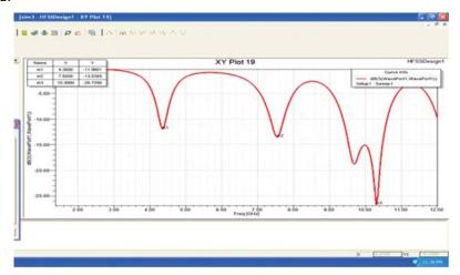
Fig 2- Return loss of slotted octagon patch antenna
