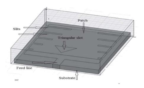
Figure 2: Isometric view of the multiband microstrip antenna
