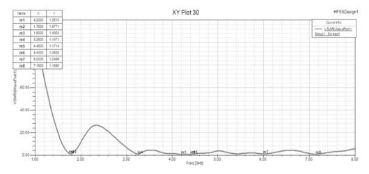
Figure 4: VSWR of Multiband Microstrip Antenna
