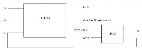
Fig 4: Block diagram of reversible triggered flip-flop
