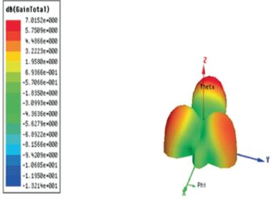
Fig 6-Gain at frequency 10.34 Ghz
