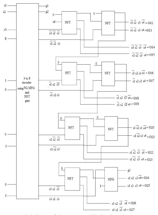
Figure 15: Block diagram of the 3 to 8 reversible decoder with FG,NFT,MFG gates
