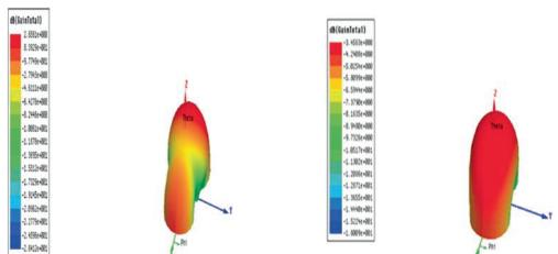
Fig-11 Gain at frequency 6.60 GHz
