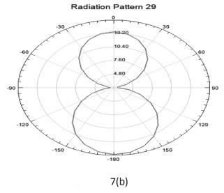
Fig. 7 (a) Radiation pattern at 5.6 GHz and (b) Radiation pattern at 7.3 GHz using roger  $\,$
