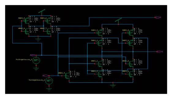
Figure 5: Circuit diagram of Feynman gate
