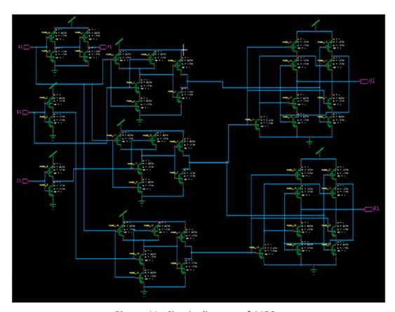
Figure 11: Circuit diagram of MFG gate
