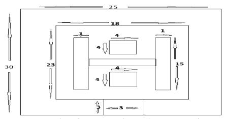
Fig. 1. Slotted antenna with H and two Square slots
