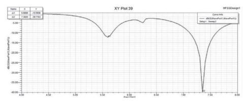
Fig. 5 Return losses using Roger RT/duroid 5870
