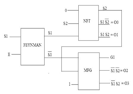
Figure 13: Block diagram of the 2:4 reversible decoder with FG,NFT and MFG gates
