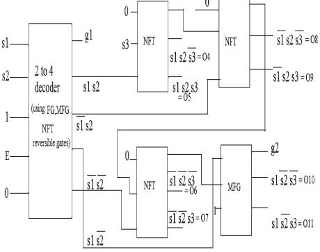
Figure 14: Block diagram of the 3 to 8 reversible decoder using FG,NFT and MFG gates
