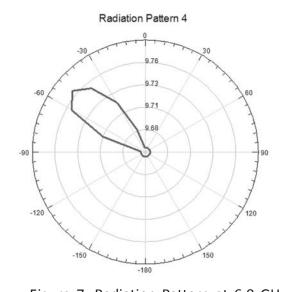
Figure 7: Radiation Pattern at 6.0 GHz
