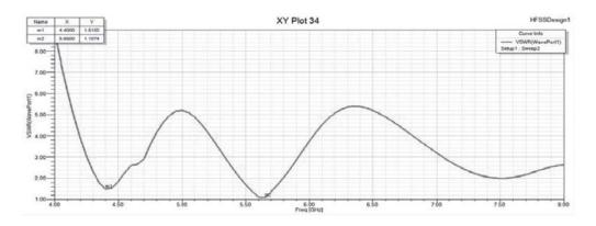
Fig.3 VSWR are on 4.4 and 5.65 GHz using FR4
