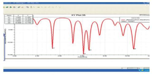
Fig 7-Return loss of unslotted octagon patch microstrip antenna VSWR 1.16 at frequency 3.35GHz , 1.44 at frequency 6.10GHz,1.55 at frequency 6.10GHz and 1.59 at frequency 10.55 GHz.
