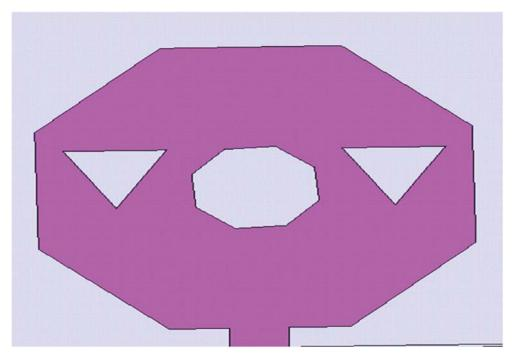
Fig 1 - Slotted patch hexagonal microstrip antenna
